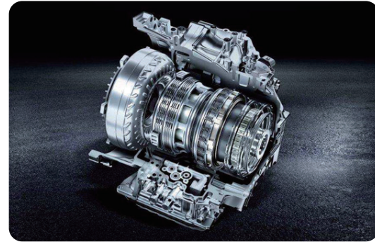
7-speed wet dual clutch transmission
